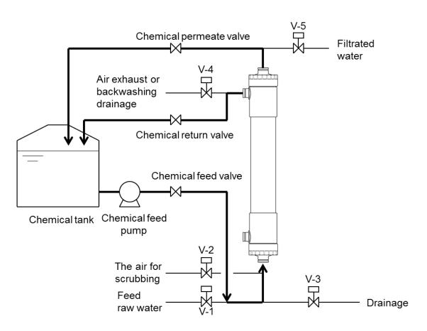
Fig. 7 Flow diagram for chemical cleaning
