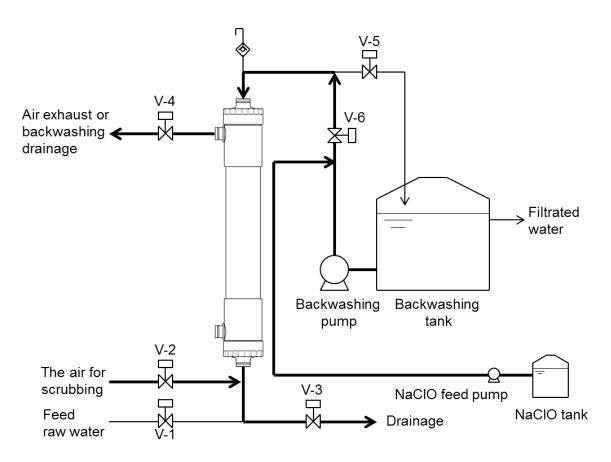
Fig. 5 Flow diagram for the TMC
