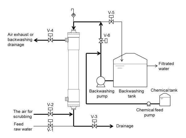
Fig. 4 Flow diagram for backwash and air-scrubbing
