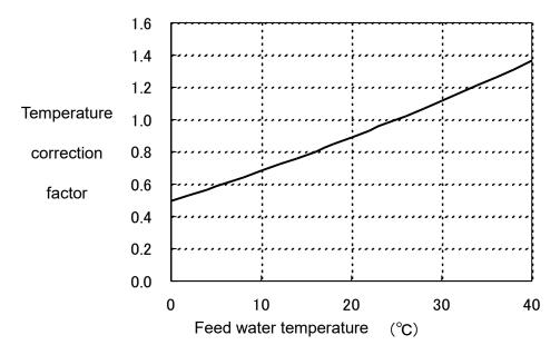
Fig. 6 Temperature correction factor (TCF)
